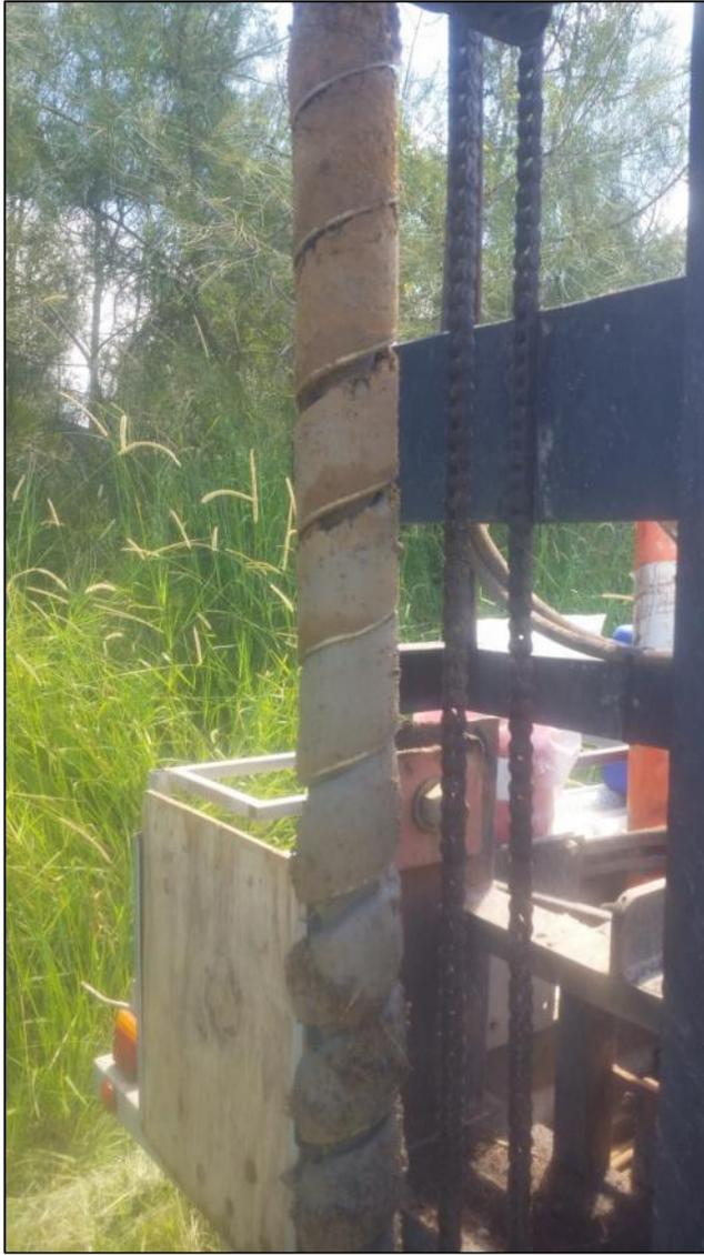
Plate 6: The typical geological profile of boreholes drilled across the site for the Acid Sulfate Soil (ASS) investigation. The profile includes silty sand profiles underlain by clay sand and sandy clay.
